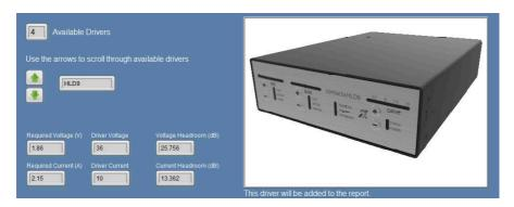
**Note:** The two sections labelled 'Voltage Headroom' and 'Current Headroom' display the amount of Current and Voltage the selected loop driver has in reserve.
