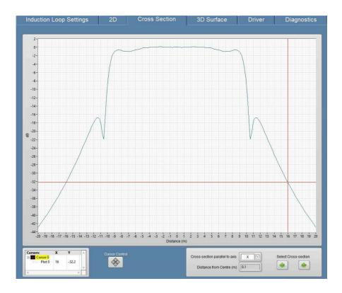
**Note:** As the scale is measured from the centre of the layout, move the vertical crosshair 10m or half the length of the X dimension of the layout, then add the distance outside the layout, 6m in this example.
